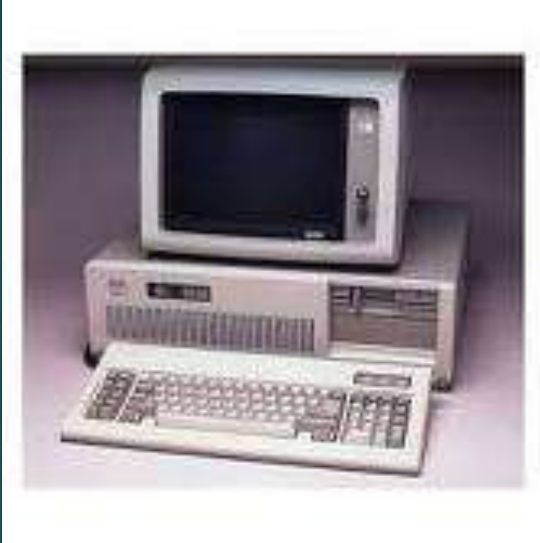
1982 IBM Computer Intel 8088 chip @ 4.77 MHz
